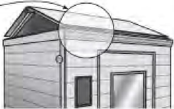
Next, take the clear plastic lining and cover the roof peak completely prior to installing the canvas cover.
