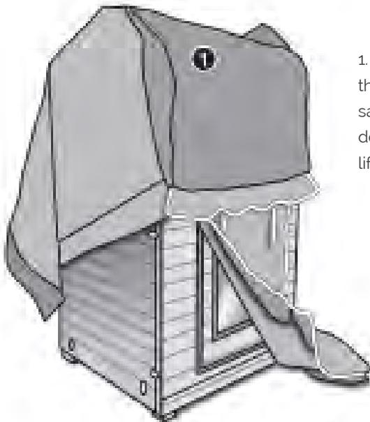
1. Take the back section of the cover and put it over the sauna. Pull the cover slowly down from the back while lifting up the front section.
