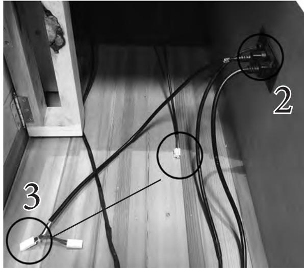
4. Lay the second bench down half way and connect the heater cable labeled "4".
