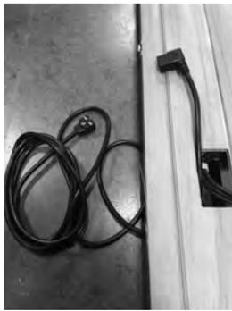
2. Push the female end of the main power cord up through the square hole in the left rear corner of the bottom.
